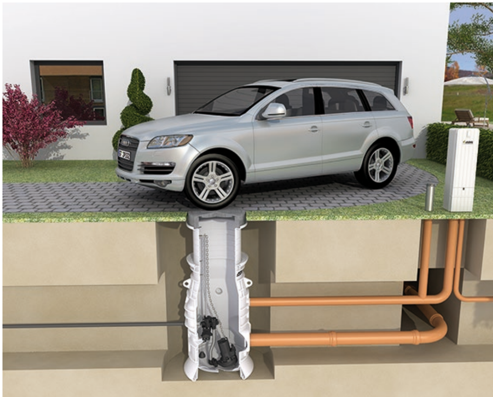
Pic 2: A pumping station in pressure drainage: The pump's cutting system ensures that solids are grinded and can be disposed of with the wastewater via small-dimensioned pressure pipes.
