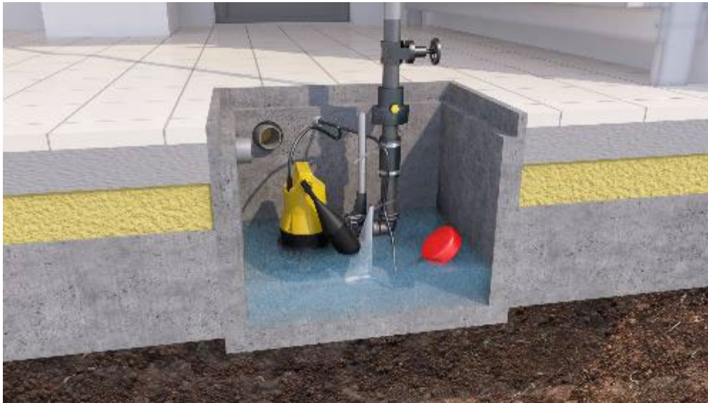
Pic 2: In addition to the standard application in basement drainage, the pumps are used for the disposal of surface water, rainwater and the draining of pools, ponds, etc.
