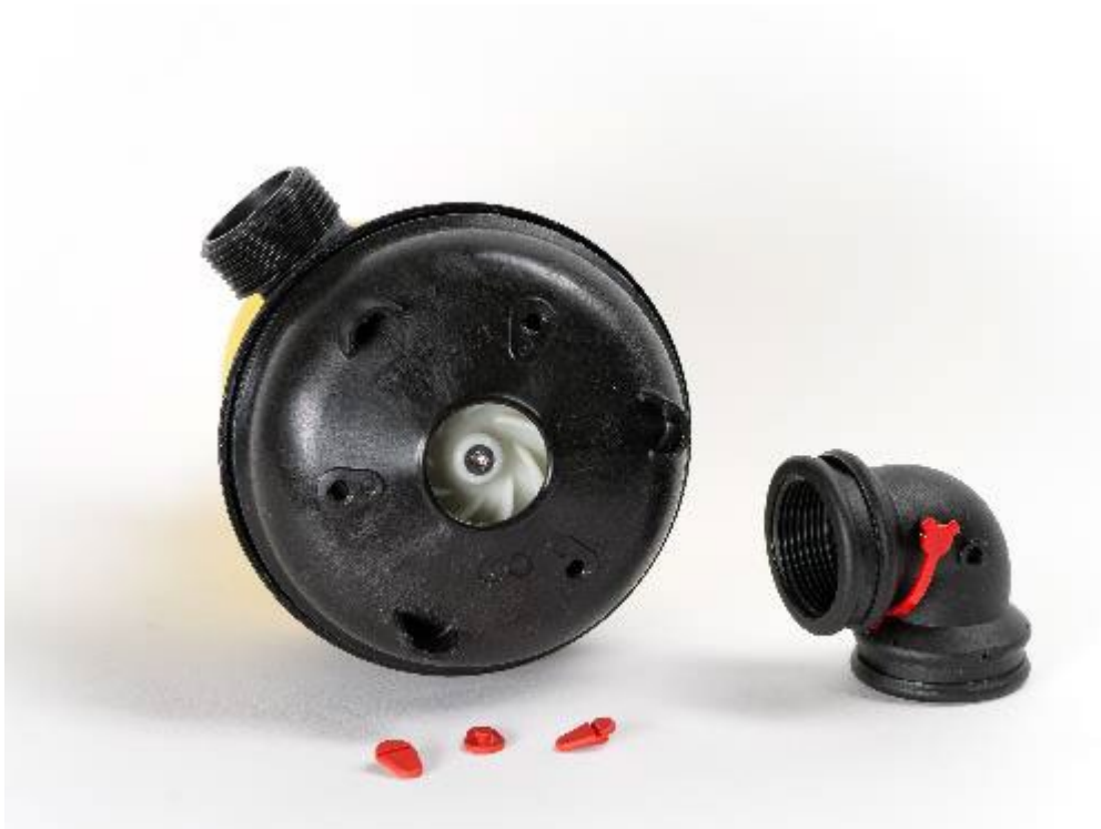
Pic 3: The flushing device for sump cleaning (at the bottom of the pump) as well as the self-ventilation (at the connection elbow) can be opened or closed without tools.
